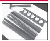
2. Align double wall vane on the two lengths of rail and press the vane into place.
