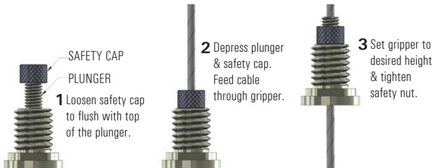
**Notes:** Minimum 2" cable to exit bottom of gripper when done.
