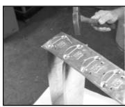
5. Align the vanes on the second length of rail and hammer over the vane, securing it to the rail.
