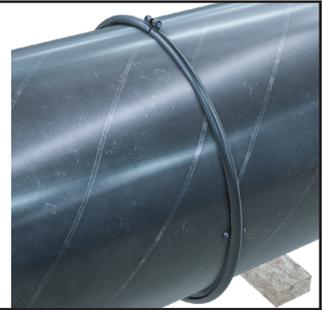
10. Tighten the bolt on the closure ring until it makes even contact around the circumference of the duct sections. Tap around joint with hammer if necessary to seat flange while tightening.
