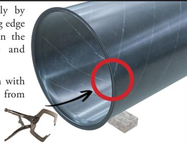
6. Complete the gasket application by installing Ductmate Neoprene gasket on the face of the flange around the entire circumference of **one** of the mating flanges.
